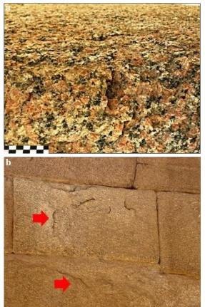
Figure (5) Shows <u>a</u>. the different minerals that make up granite <u>b</u>. separation in layers due to the variation in the physicochemical composition of the granite minerals
